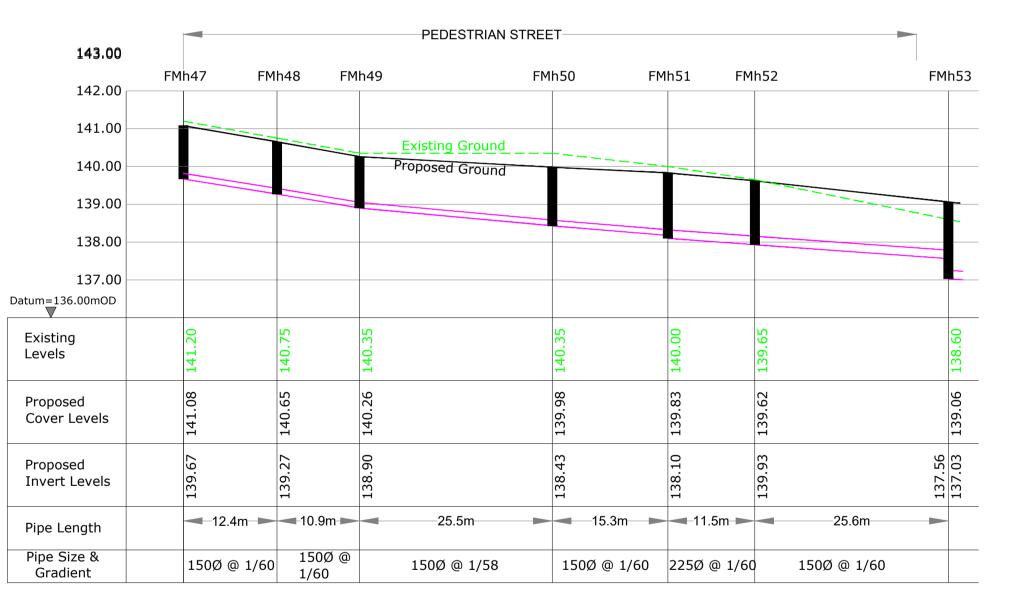
Foul Longitudinal Section FMh47 to FMh53 Vertical Scale 1:100 Horizontal Scale 1:500
